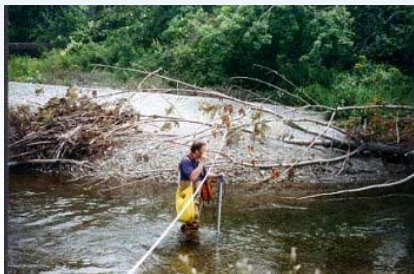
Velocity measurements across stream channel with current meter.
